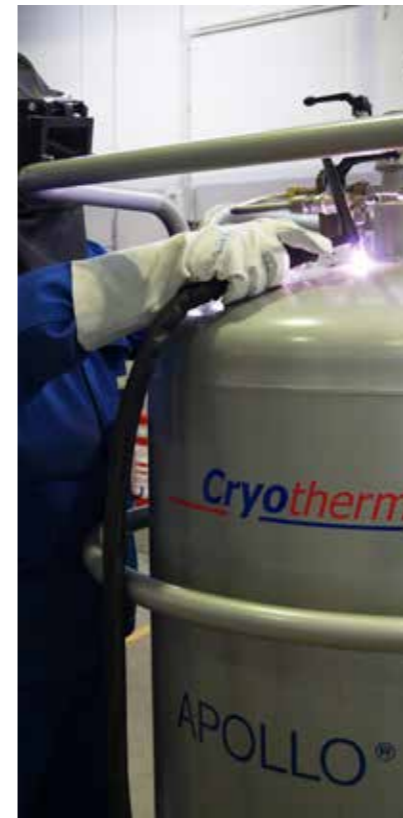
WIG welding wolfram (tungsten)-inert gas welding
