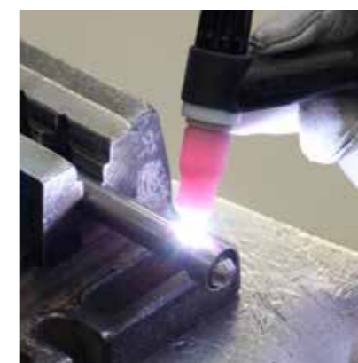
WIG welding wolfram (tungsten)-inert gas welding
